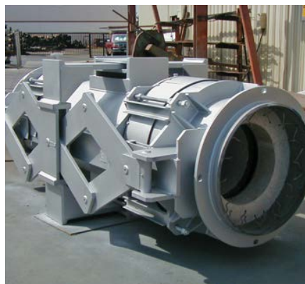
Recirculation catalyst standpipe refractory lined expansion joint (800mm ID).
