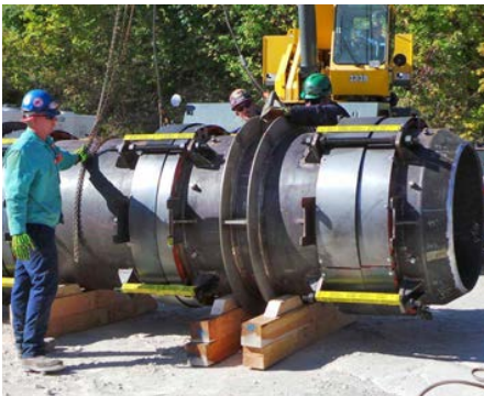
DN1400mm cold wall universal expansion joint cartridge for FCCU.
