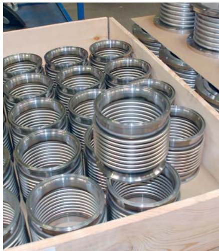
UM-types are manufactured with semi or fully automated operations for large series production.
