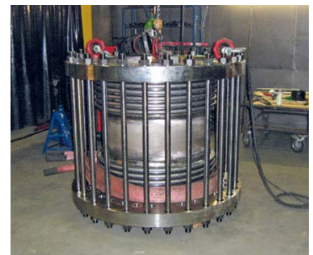
Testing a metal expansion joint with helium.
