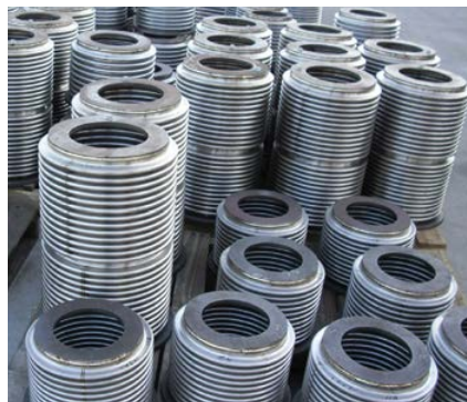
Metal pipe penetration seals.
