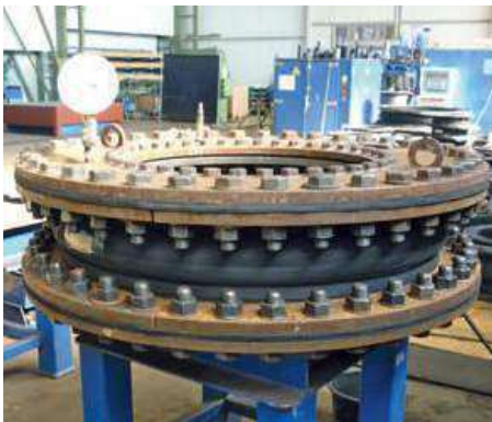
Hydraulic Pressure Testing.
